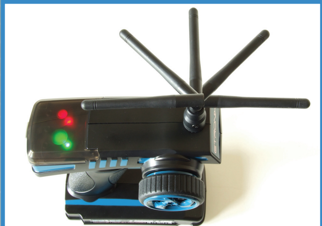
The aerial folds down for storage The aerial base also rotates 180 degrees so once you have a comfortable grip on the transmitter the aerial can be moved to the most vertical position to maximise range.
