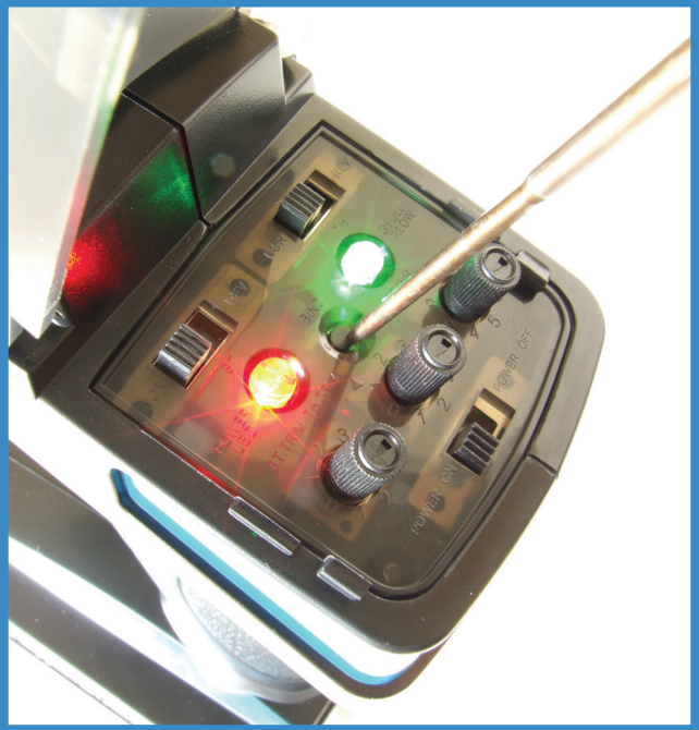
With the power on you can release the bind button once the green LED begins to flash to indicate the "Bind" process has initiated.
