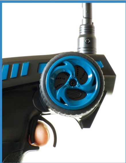
When pulled back to the handset the model should move forwards, if not flick the Throttle switch to the 'Rev' position.
