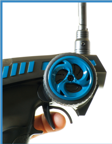
When at the mid position the model should remain stationary, if it creeps slightly adjust the throttle neutral dial accordingly.
